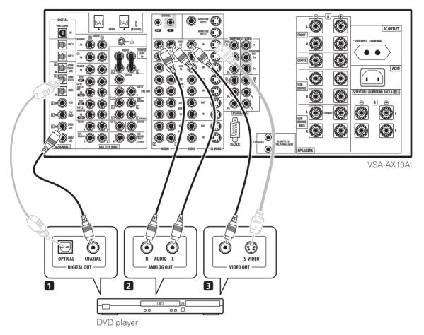
Different DVD players offer a different selection of connections, but all should give you at least a digital audio output, stereo analog audio outputs and a video output. Additionally, you may have a player with multichannel analog audio outputs and different kinds of video outputs to choose from.
